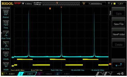
Linewidth measurement using Fabry-Perrot Interferometer
